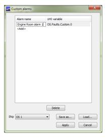
4. To change the UHI-variable value, double-click on the value in the **UHI variable** column, and select a new value from the drop-down list.
