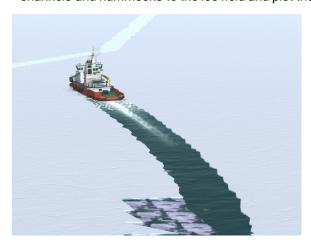
Method 2: Creating the ice zone by using the Ice generator object of the Environment category (see "Using Ice Generator Object" on page 351).
