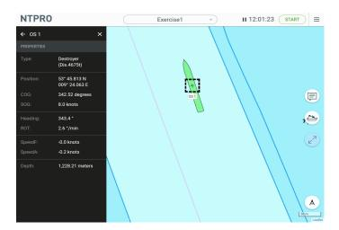
The following ship properties are displayed in the **PROPERTIES** list: type, position, COG, SOG, heading, ROT, fore/aft speed, depth.
