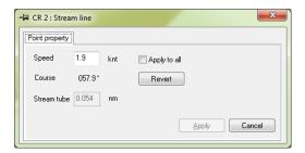
2. In the Speed field, set the stream speed at the start point of the segment (default speed is 1.9 knots).
