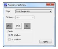
3. To cancel the generator fault, clear the checkboxes on the Auxiliary machinery panel and click the Apply button.
