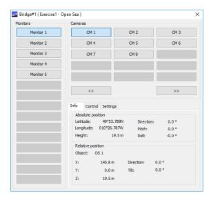
NOTE: If the monitor is selected, any successive clicking on the camera button will result in this camera reassignment to this monitor. The same camera can be assigned to several monitors.
