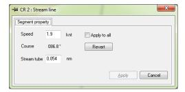
4. In the Speed field, set the stream speed on the selected segment of the stream line.
