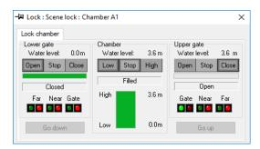
5. After the ship has entered the lock chamber, click the Close button to close the upper gate .
