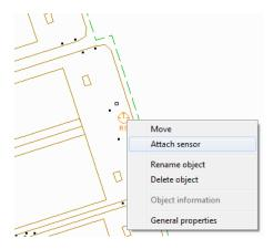
4. Click on any point on the barge. The sensor is attached to this barge.
