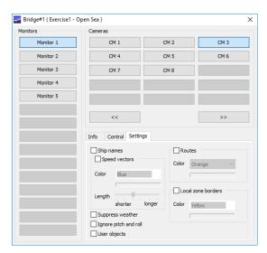
4. To display the ship names (above the ships) on the Instructor visualization screen, select the **Ship names** checkbox.
